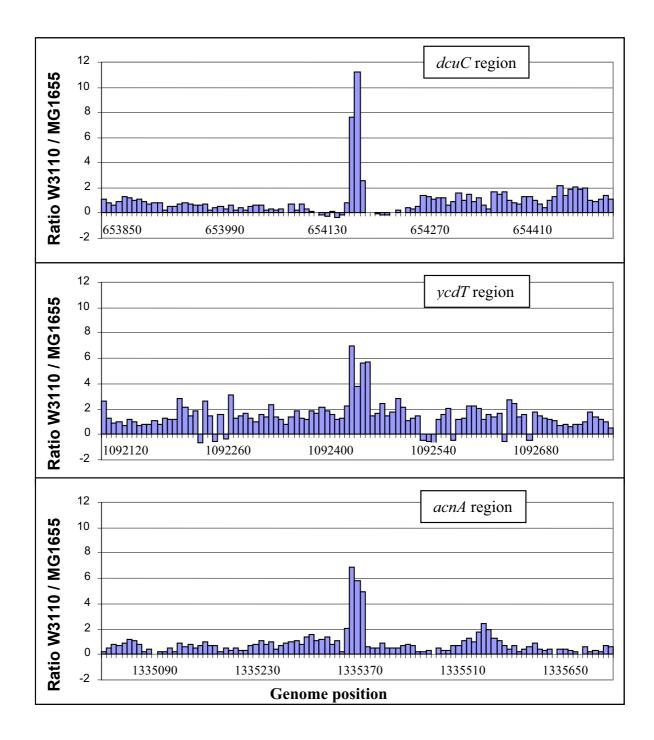
**Figure 1**Sample mutation mapping data. The ratio of signal of W3110 vs. MG1655 is shown for probes spaced every ~7 bp surrounding an IS5 insertion in *dcuC* (top), a SNP in *ycdT* (middle), and a SNP in *acnA* (bottom).
