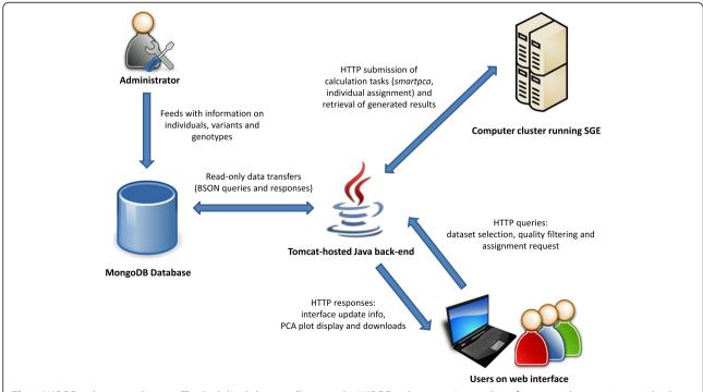
Fig. 1 WIDDE architecture diagram. This high-level diagram illustrates the WIDDE architecture. It provides information about entities involved when using the information system, the data flows that occur between them, and the third-party software used in the process
