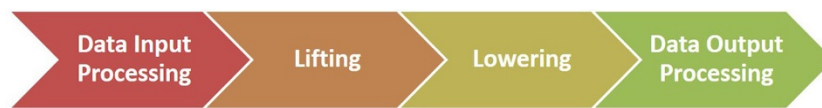
Figure 7 Connector implementation functional blocks. An arrow represents an implementation functional block. The left to right serial disposition of the arrows indicates the order in which each functional block should be executed, starting at the Data Input Processing block.
