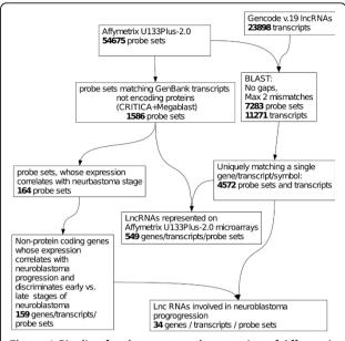
**Figure 1 Pipeline for the automated annotation of Affymetrix U133 IncRNAs.** Blocks represent data sets emerging from the analysis and rules used for their generation. Numbers represent the number of entries in each dataset.
