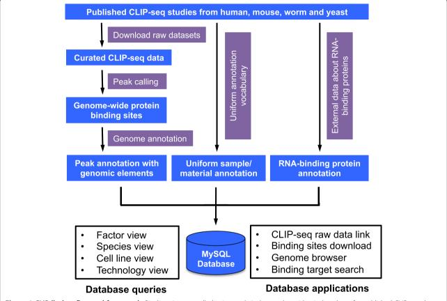
**Figure 1 CLIPdb data flow and framework.** Binding sites are called using analytical procedures identical to those for published CLIP-seq data sets. Additional information about the CLIP-seq data sets and RBPs are collected from external databases. All metadata are organized for convenient queries and applications. The details are described in the Construction and Content section.
