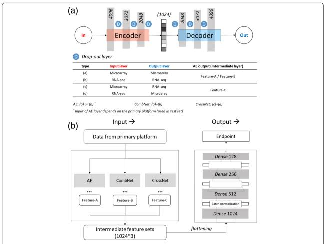
Fig. 2 HetEnc overview. (a) feature representation model architecture and three different encoding networks (AE, CombNet and CrossNet) used in the study; (b) feature extraction and 6-DNN structure in the modeling step
